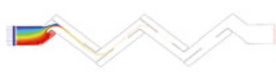
حذف 99% قطرات و ذرات Elimination of 99% of droplets and particles
