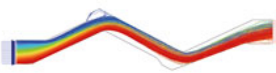
حذف 30% قطرات و ذرات Elimination of 30% of droplets and particles
